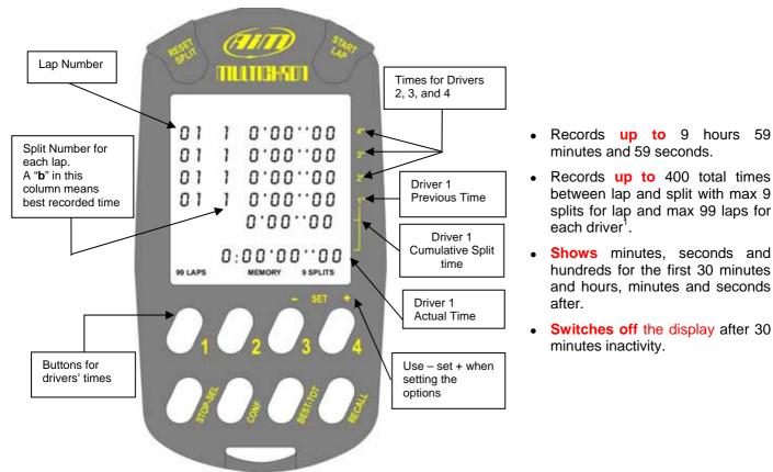
**Multichron** is the handheld *AIM* "multi-chronometer" that lets you time up to four drivers simultaneously. You can time and record up to 99 laps (with up to 9 split times for each lap) for each driver. **Multichron** is a flexible instrument that fits any racing situation with two start modes (**Multi Start** and **One Start**) and two recording modes (**Multi Key** and **One key**).
