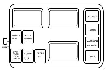
Use the buttons on the left side of the DT-32K5 to turn the instrument on and off.
