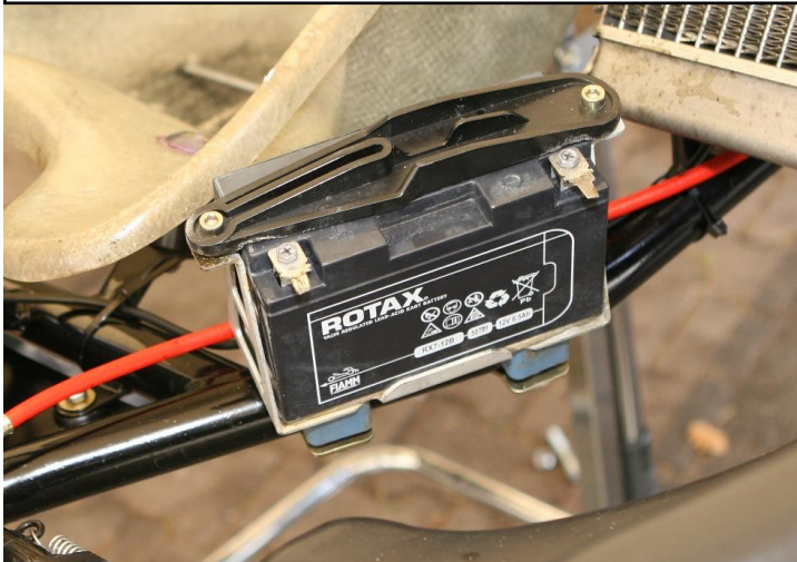
Lead acid battery, mounted on Chassis
